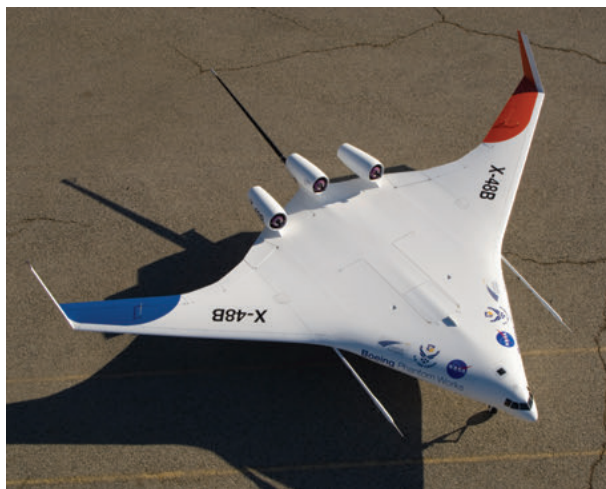
Modern CFD has revolutionized wing design. The Boeing Blended Wing Body is in design for the year 2020 or sooner.
