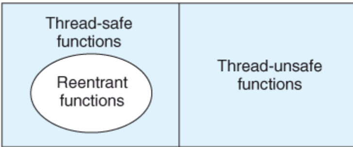
Figure 12.39 Relationships between the sets of reentrant, thread-safe, and thread-unsafe functions.
