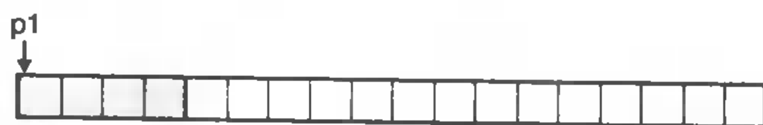
(a) p1 = malloc(4*sizeof(int))
