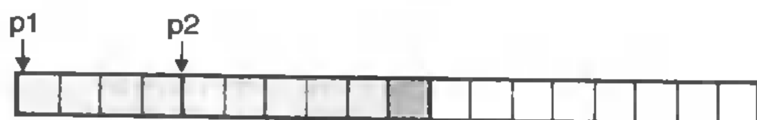
(b) p2 = malloc(5*sizeof(int))
